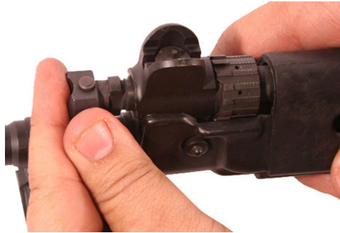
Figure 9. Installing the Gas Plug.
