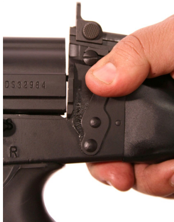
Figure 1. Separating the Receivers.
