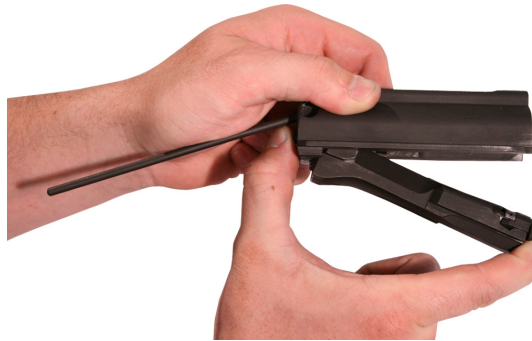
Figure 10. Inserting the Bolt Assembly into the Breech Block.
