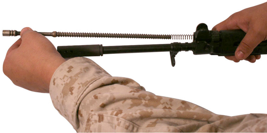
Figure 7. Removing the Gas Piston and Gas piston spring.
