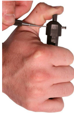
Figure 5. Removing the Firing Pin Retaining Pin from the Bolt.
