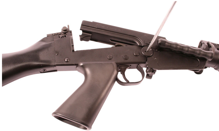
Figure 12. Installing the Takedown Screw.
