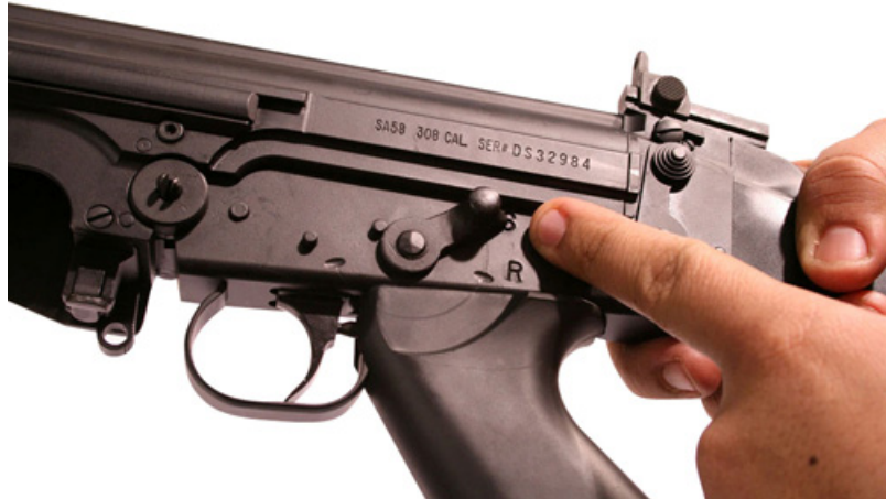
Figure 6. Selector Lever on SAFE.
