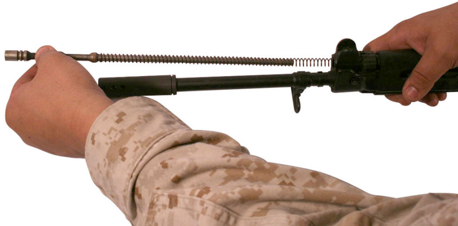
Figure 8. Inserting the Gas Piston and Gas Piston Spring into the Gas Tube.
