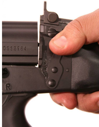
Figure 9. Pulling the Takedown Latch to the Rear.
