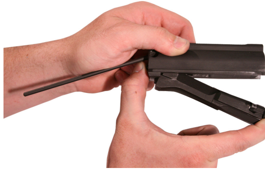
Figure 4. Removing the Bolt Assembly from the Breech Block.
