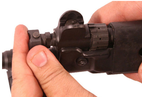
Figure 6. Removing the Gas Plug.
