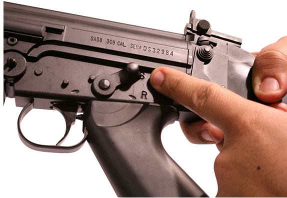
Figure 2. Selector Lever on SAFE.
