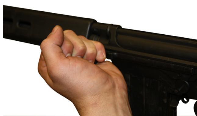
Figure 1. Pulling the Charging Handle to the Rear.
