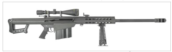
Ronnie Barrett's M82 (c. 1982) anti-material rifle is chambered for the .50 BMG round first used in the Browning M1918 heavy machine gun. It was adopted by the US Army in 2003 (as the M107).
