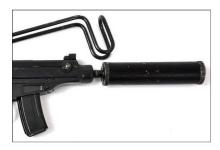
Most .32 ACP rounds are subsonic, thus very well suited to covert use when fitted with a silencer like the one pictured, which is similar in size to the Omega 45K from Silencer Co.
